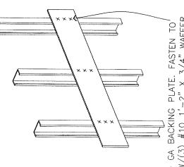
6" X 20 GA BACKING PLATE. FASTEN TO<sup>1</sup> STUDS W/(3) #10 1'-2" X 3/4" WAFFER HEAD SELF DRILLING SCREWS PER STUD. ALL BACKING TO SPAN MIN OF (3) STUDS. BACKING PLATE TO BE Fy=50KSI A PLATE BACKING
