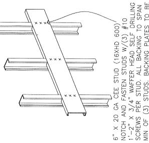
MIN OF (3) STUDS. BACKING PLATES TO BE Fy=50KSI STEEL B STUD BACKING 6" X 20 GA CEE STUD (16XHD 600)
