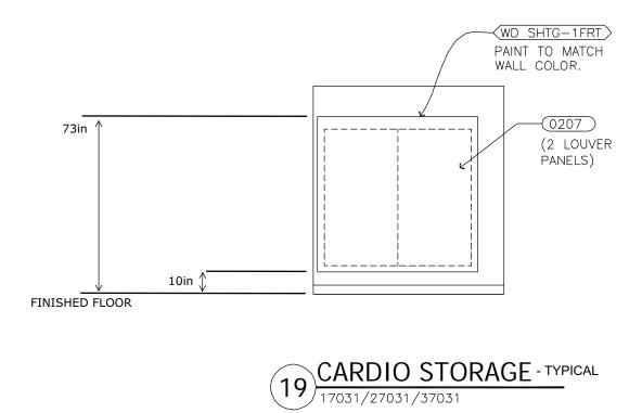
**INSIDE WALL BACKING DETAIL** START 10in FROM FINISHED FLOOR 73in FROM FINISHED FLOOR END
